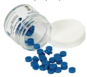
The Economy **diskobolus™** Blue septa are designed for non-demanding, routine applications. They are easy to penetrate, with a durometer rating of 40-45. These septa can be used up to 200-250°C and are suitable for 90% of all GC analysis. Made from silicone. The package is for 100 pieces.
